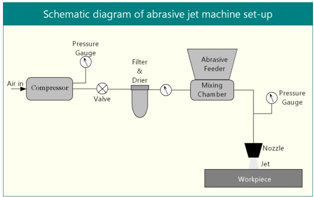
Figure a- Schematic diagram of Abrasive jet machine
